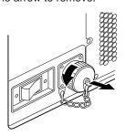
2. Insert the projector plug of the supplied power cord into the power input terminal of the projector.
